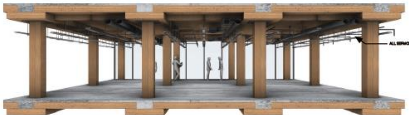
CLT / Concrete Composite System Full CLT structure acts as formwork for concrete screed and beams
