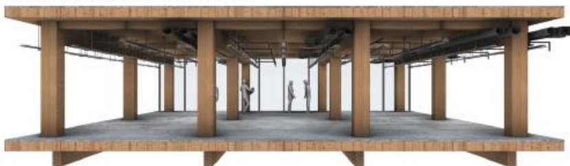
CLT / Concrete Composite System Full CLT structure acts as formwork for concrete screed and beams
